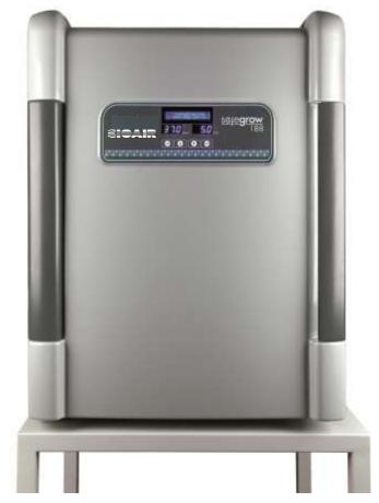
The accuracy and precision of the temperature are ensured by 4 direct, validated and independently controlled heating elements, positioned on the 6 sides of the chamber, capable of measuring and controlling the temperature with a difference of 0.1 degrees with respect to the fixed value. There
